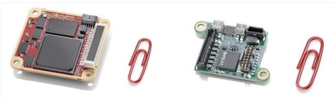
FIGURE 5: The VX1000 measurement hardware is connected to the control unit via a compact POD (Plug-On Device).
