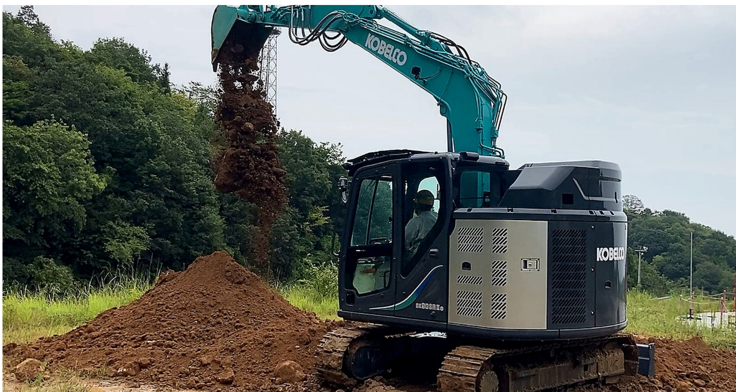
A battery-powered electric hydraulic excavator developed by Kobelco
