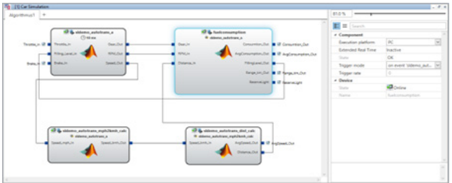
Figure 1. For calculations of necessary data, CANape's function is used to calculate data obtained with CSM modules. It is realized by combining several subfunctions.
