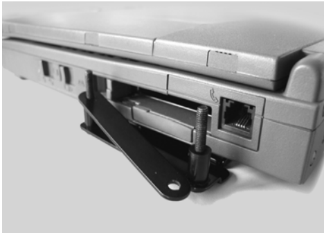
Fig.9: Adjust the clamping plate with spacers as needed
