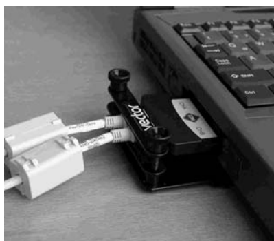
Fig.15: This is needed if the pcmcia card / cardbus card is longer than the slot.
