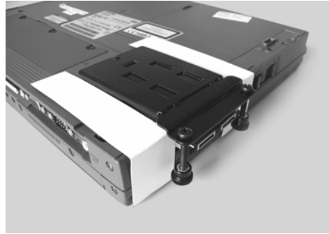
Fig.4: Press the Cardsafe to the bottom of the notebook in the opening of the template.
