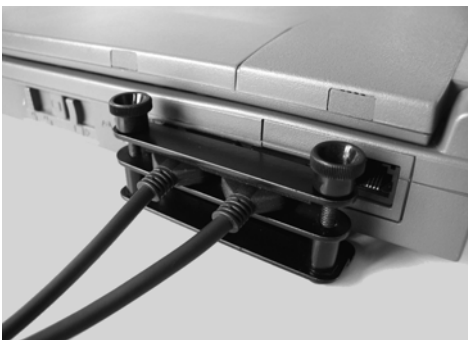
Fig.11: Fix the clamp plate with knurled nut.
