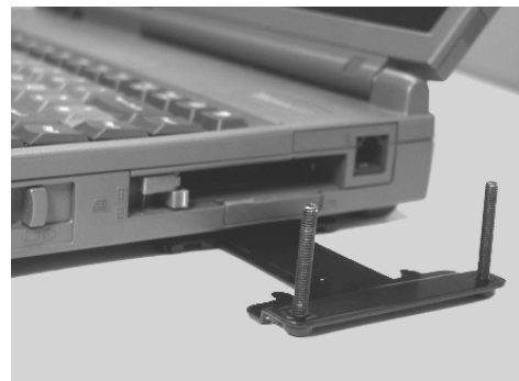
Fig.8: plug in the connector fixture.
