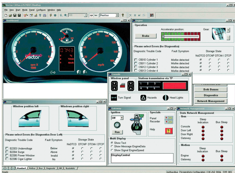
Figure 6. CANoe panels for controlling ECUs. Courtesy of Vector CANtech.
