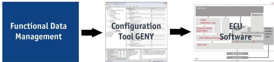
[Figure 2: Code for the ECUs is generated based on the description of the electronic structure in eASee's functional data management.]
