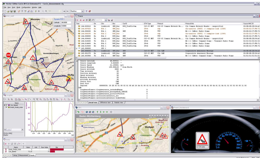
[Figure: CANoe.IP simulates a traffic scenario; this example is based on a traffic jam warning that is received.]
