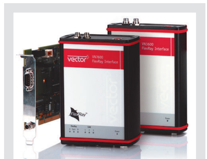
Figure 4: VN interfaces from Vector fulfill the strict bus interface requirements imposed by the FlexRay bus. The USB variants VN3600/VN7600 are suitable for mobile applications, analyses and simple simulations. The PCI variant VN3300 supports complex simulations of multiple ECUs with real-time requirements.
