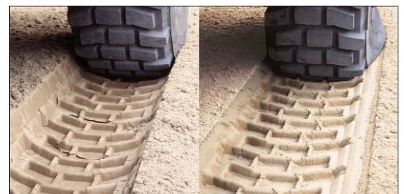
■ Figure 2. Tire pressure control while driving is possible, e.g. to avoid site damage.
