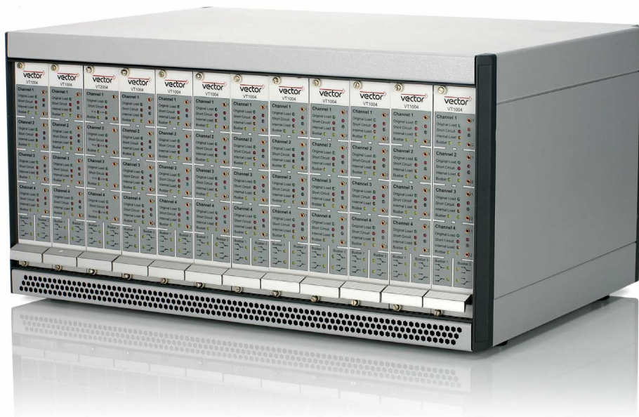
[Figure 3: The VT System consists of standard 19-inch housings with their own backplane into which the modules are inserted. This lets users implement individual and flexible test solutions depending on requirements.]
