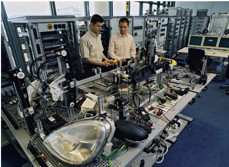
[Figure 3: Electronic components for the A-Class vehicle are tested on an integration test bench]
