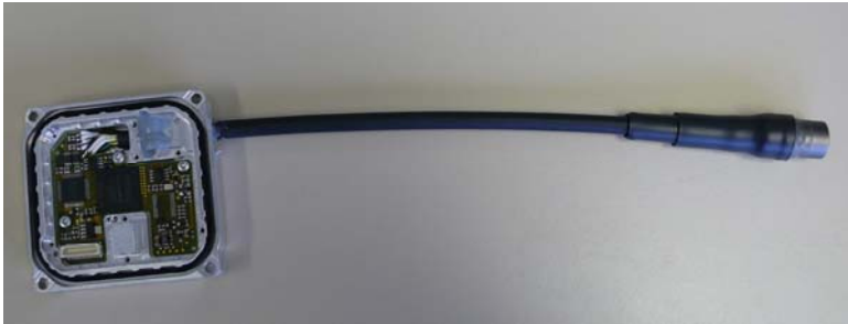
Customized POD in ECU cover-plate (waterproof)
