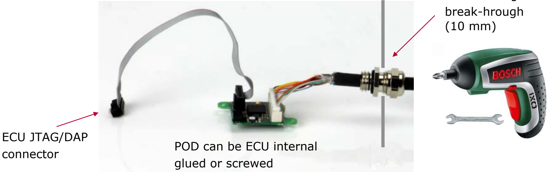
POD ECU internal mounted
